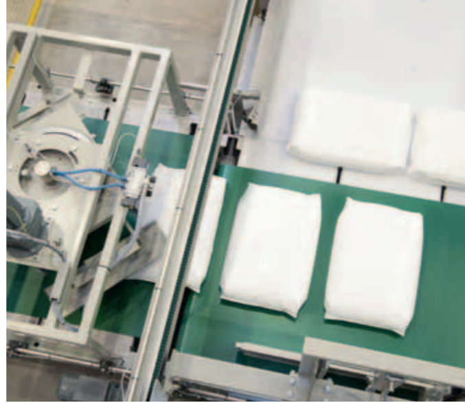
02. Gentle Bag Formation | Layers of packed goods are gently positioned according to the individually specified layer pattern.
