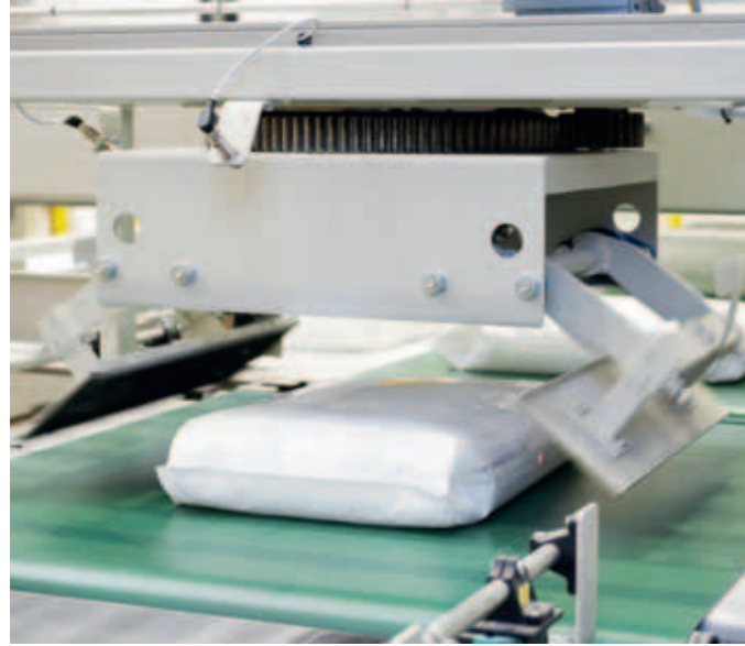
01. Low Bag Infeed | The low bag infeed allows to overview the complete work process.
