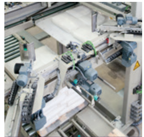
► Layer formation, packaged goods formed length-wise and width-wise and positioned.
