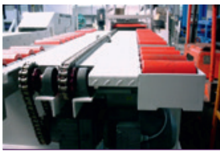
▶ Combined chain roller track for pallet transport
