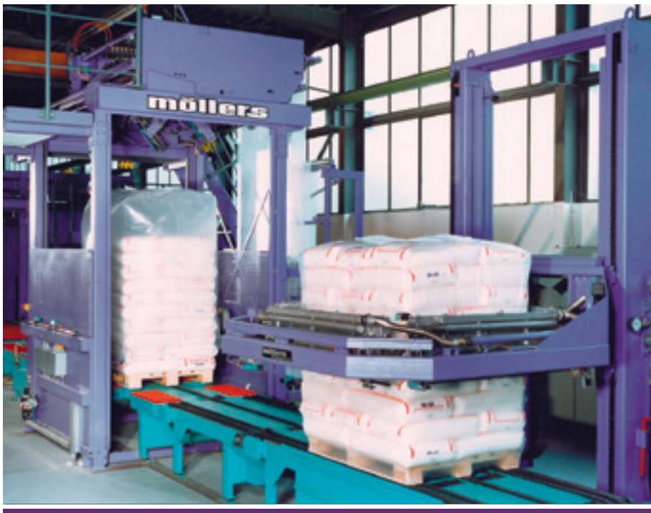
► FSA tubular film drawing machine with downstream SR shrink frame
