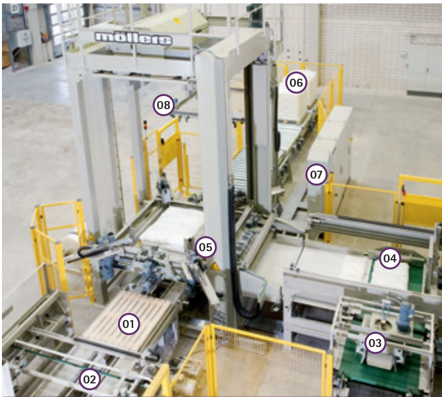
► 2in1 palletizer with stretch-hooder ► 01 Feed for empty pallets, 02 Flat-film positioner, 03 Low entry for the packed goods, 04 Palletizing according to customer specifications, 05 Load security at same point, 06 Pallet ready for transport, 07 Easy handling via a central operating element, 08 External infeed with contour check and pallet centralizing (also for Octabin, FIBC etc.)
