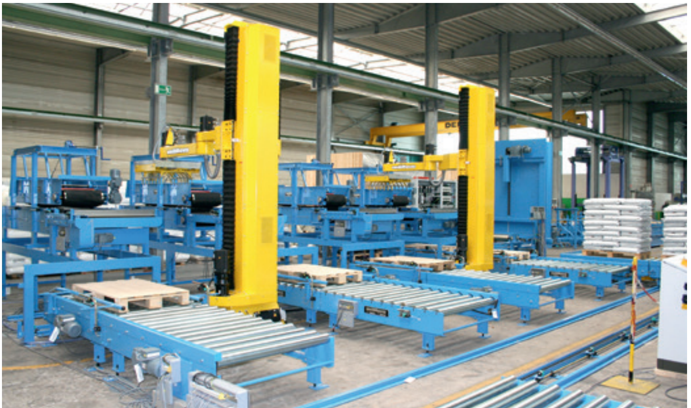
► Romeo® palletizer robot shows 4 lines simultaneously with decentralized empty-pallet feed
