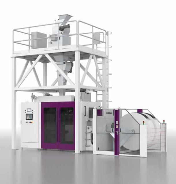
Möllers Packaging Technology GmbH (MPT) presents the new high-speed Form-Fill-Seal system (HSB-2600) for plastic granules with a fill weight from 5 to 50 kg. It offers a unique system concept to maximise resource efficiency while keeping the production quality at the maximum for up to 2,600 bags per hour. The HSB-2600 produces space-saving and material-saving bags. Corner welding is utilised to create brick-shaped bags which are ideal for stacking on pallets.
