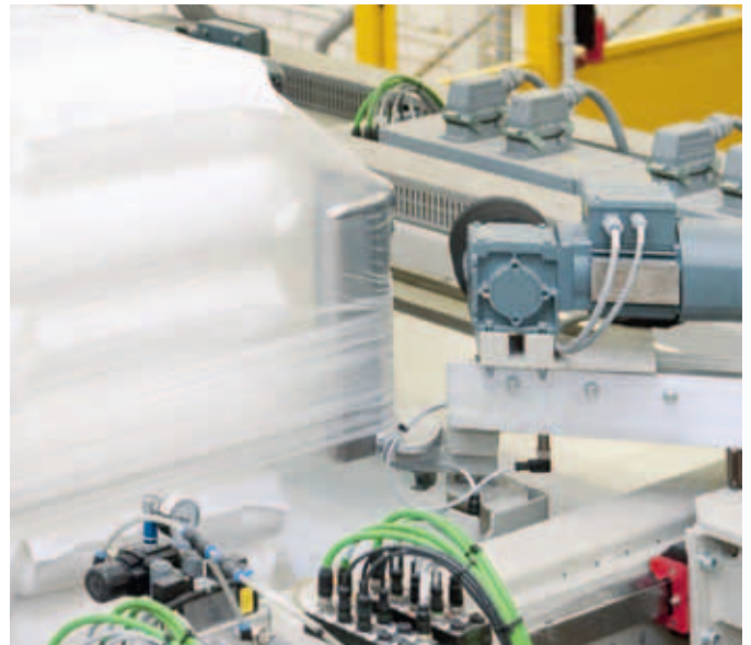
11. Film Wrapping | High reset forces for a secure load on the pallet.
